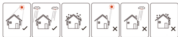
Fig. 7. Recommended locations for the inverter and batteries.
