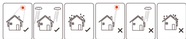
Fig. 13. Recommended locations for the inverter.
